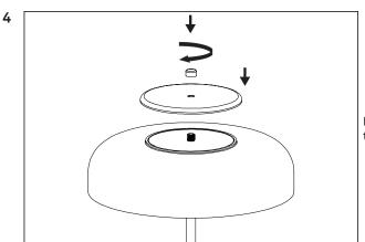
Place the cover plate back on top and tighten the finger screw.
