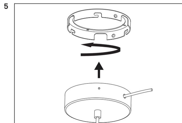
Attach the ceiling plate to the top plate by turning the ceiling plate.
