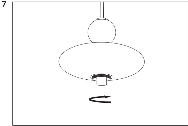
Screw the light bulb into the socket.
