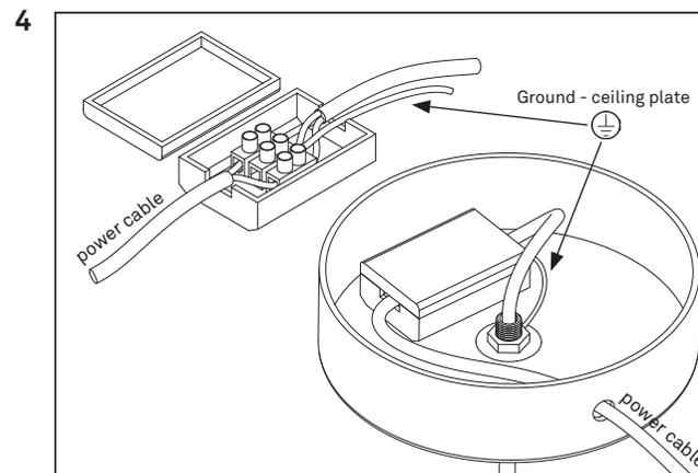
Install the power cable by leading it through either the top or the side of the ceiling plate through the cable relief and into the cable connector. Please make sure the cable relief is tightened.
