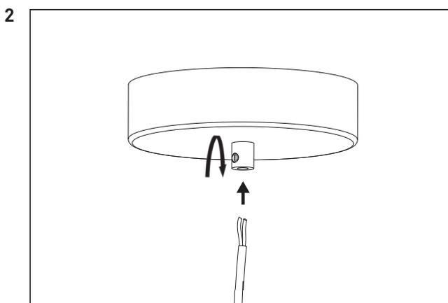
Lead the fabric cable in through the cable relief at the bottom of the ceiling plate. Adjust the cable to the desired length. Be sure to tighten the screw carefully and to leave enough of the cable inside the ceiling plate so the end can reach the cable connector.
