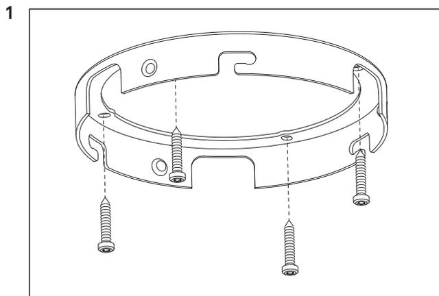
Mount the top plate to the ceiling with screws.
