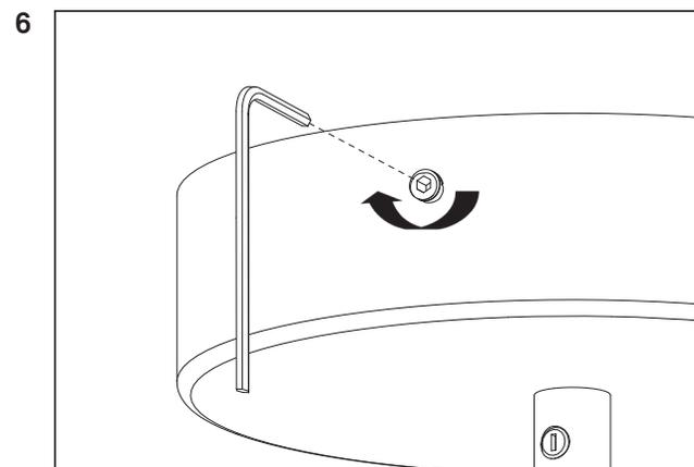
Fixate with the socket screw. Install the socket screw with the Allen key provided.
