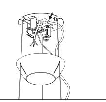
Pull the lamp cable through the cover plate and the strain relief.
