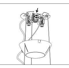
Connect the wire-ends of both the power cable and the lamp cable to the cable terminals. Match the brown wire with "L" the blue wire with "N" and the green/yellow wire with the grounding symbol.
