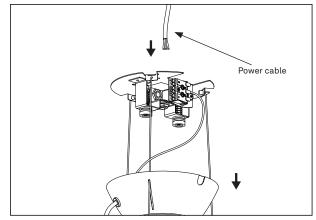
Pull the cover plate away from the mounting bracket. It is attached with strong magnets and might require some force. 4
