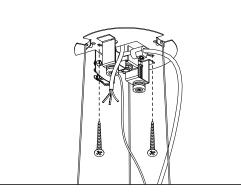
Attach the mounting bracket to the ceiling.
