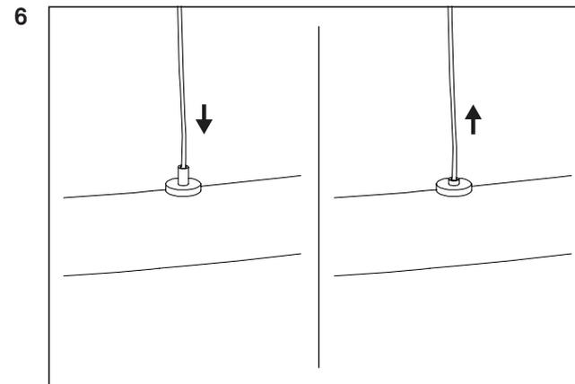
Adjust the lamp to its final position. It is recommended to use a spirit level.
