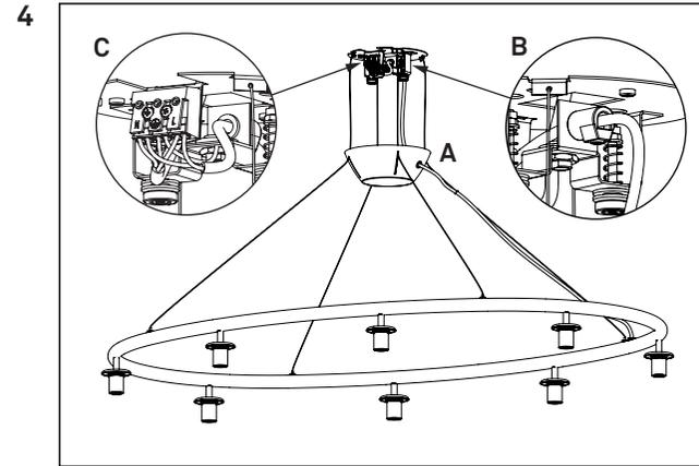
Push the lamp cable through the cover plate (A) and strain relief on the mounting bracket (B). Connect the cable-ends to the cable terminal (C).
