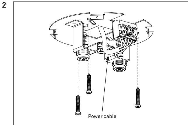
Attach the mounting bracket to the ceiling.
