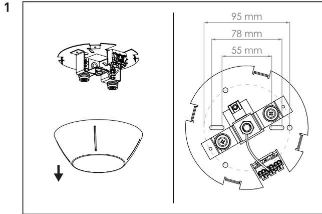
Pull cover plate away from mounting bracket. It is attached with strong magnets and might require some force.
