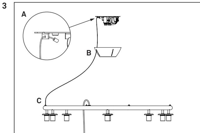
Lead the suspension wires through the mounting bracket (A), cover plate (B) and into wire lock on the ring (C). The wire locks automatically prevent the wire from coming out.
