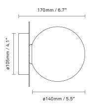
**Liila 1 Outdoor** is an extension of the Liila collection, designed to be suitable for the entrance areas of a home. A thin round sheet of metal in a dark bronze powder coating comprises the base and is topped with an opal white glass globe from which a soft, evenly diffused light is spread. Illuminate every entrance of the home with Liila 1 Outdoor and create a warm welcome.
