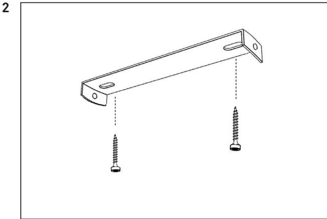
Mount the bracket to the ceiling with screws.
