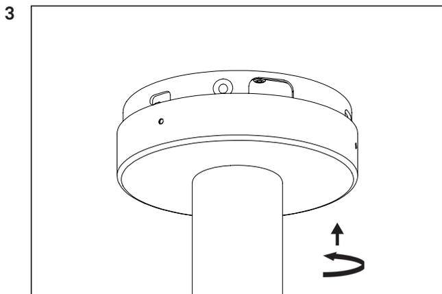
Push the lamp up into the ceiling bracket and turn against the clock to fixate in place.
