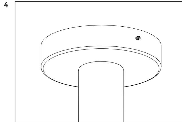
Lock the lamp in place by tightening the set screw with the included allen key.
