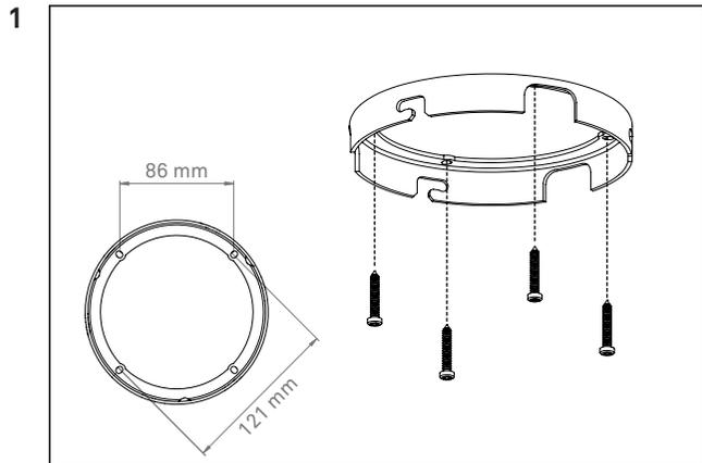
Mount the ceiling bracket to the ceiling with screws.
