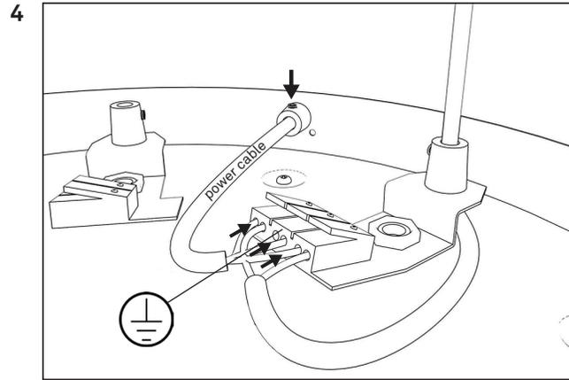
4 Lead the power cable into the ceiling plate and make sure the cable relief is tightened.
