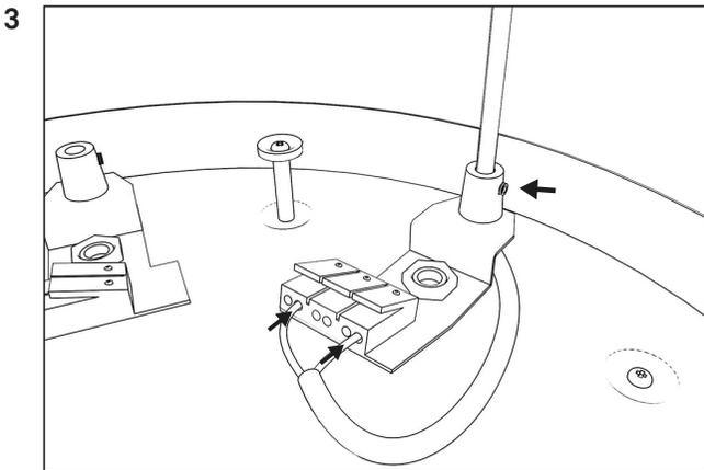
3 Lead the cables through the cable relief and fixate the cable by turning the screw clockwise.
