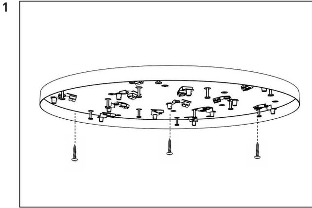
1 Fixate the mounting plate to the ceiling with screws.
