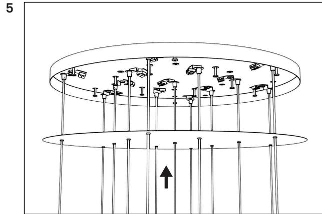
5 Attach the cover plate to the ceiling plate by carefully sliding it up and let the magnets fixate the cover plate to the ceiling plate.
