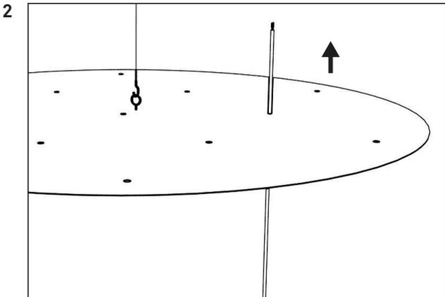
2 Lead the cables through the cover plate.
