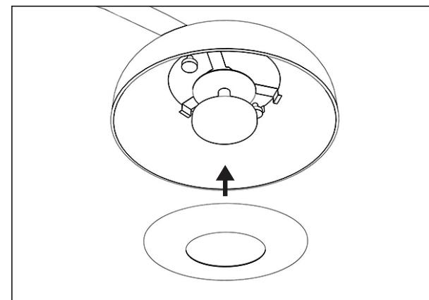
Attach the inner plate by carefully sliding it up and let the magnets fixate the plate to the lamp.
