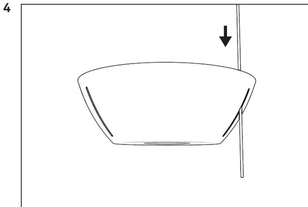
Lead the wires through the top of the cover plate.
