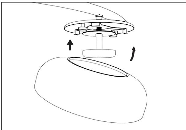
Attach each glass by fixating them with the three hooks located inside each of the 8 lamps.
