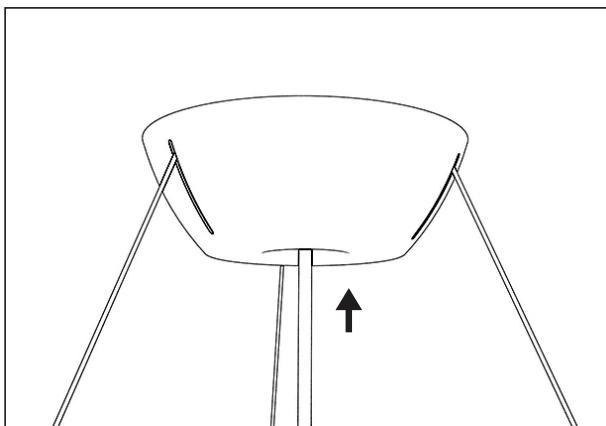
Attach the cover plate to the mounting plate by carefully sliding cover plate up and let the magnets fixate it.
