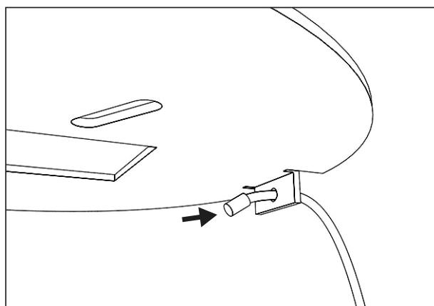
Lead the three wires through the holes in the mounting plate.
