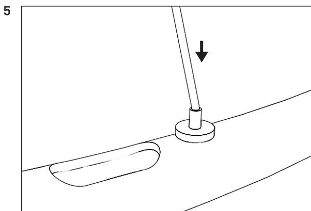
Lead the wires through the three wire locks on the ring. The locks will automatically keep the wires in place.
