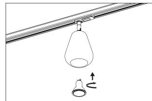
Place a GU10 light bulb in the socket by inserting it and twisting clockwise. The bulb is NOT included.
