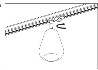
Lock the lamp in place by turning lock to the center position.
