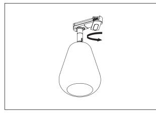
Turn the lock to be able to place the adaptor into the track.
