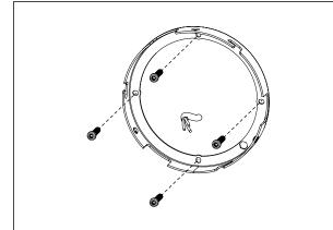
Mount the bracket to the wall or ceiling with screws.
