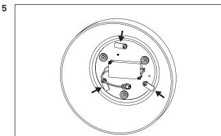
Place the glass on the base and turn the plates to hold it in place.
