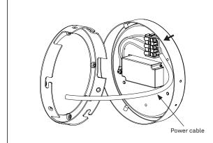
Connect cable ends to cable terminal. Match the brown wire with "L" the blue wire with "N" and the green/yellow wire with the grounding symbol.
