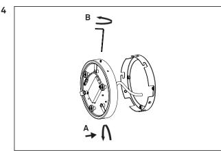
A: Attach the base of the lamp to the bracket by aligning the pins inside the base with the slots in the bracket and twist the base counterclockwise.
