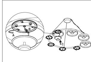
A: Place glass on lamp base and turn the three locks to hold it in place.
