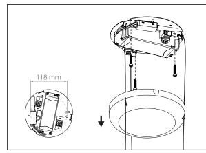
Remove the cover on the canopy. Magnets hold the cover in place.
