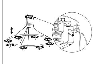
Roughly adjust the lamp height. Lock in place with the wire locks. The final position will be adjusted as the last step of the installation process.
