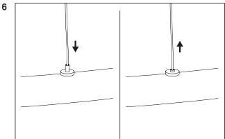
Use the wire locks on the ring to adjust the lamp to its final position. It is recommended to use a spirit level.
