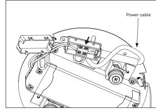
Lead the power cable through the hole in the mounting bracket and into the connector
