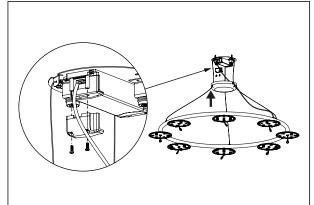
Shorten the lamp cable if necessary and connect it to the secondary (low voltage) side of the driver.
