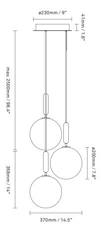
Miira 3 Large in brass finish with mouth-blown optic clear glass. Incl. Ceiling plate.
