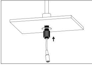
Place the washer and the hand screw over the cable and tighten against the mounting surface.
