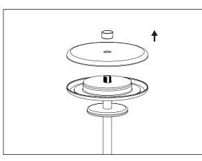
Unscrew the finger screw on top of the lamp and remove the cover plate.
