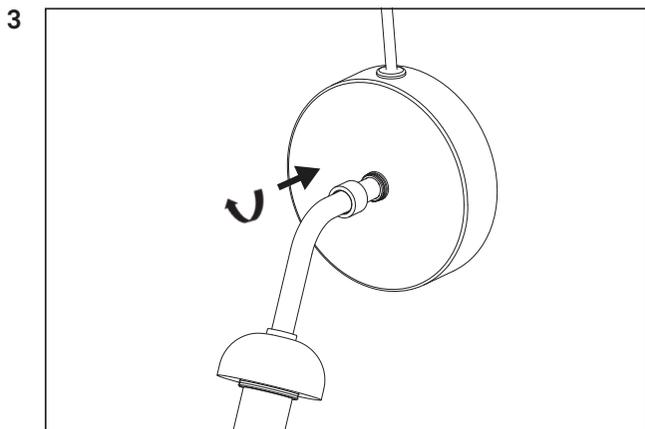
3 Turn the cover plate to align cable in desired direction.
