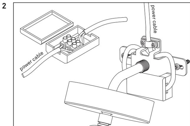
2 If the power cable is surface mounted make sure to put the cable through the hole in the cover plate before the following,
