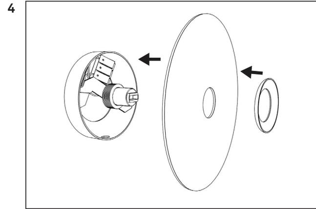
Carefully place the cover plate over the socket. Afterwards place the small metal plate over the socket.
