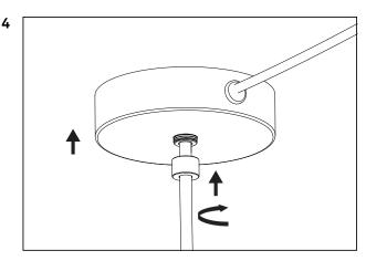
Turn the cover plate to align cable in desired direction.
