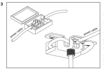
If the power cable is surface mounted make sure to put the cable through the hole in the cover plate before the following,
