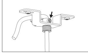
Adjust the height of the lamp by pulling the cable through the cable relief.
