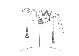
Mount the ceiling bracket to the ceiling with screws.
