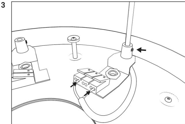
Lead the cables through the cable relief and fixate the cable by turning the screw clockwise.
