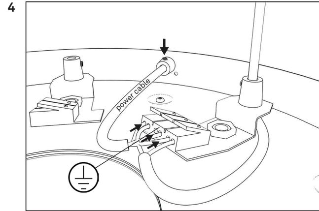
Lead the power cable into the ceiling plate and make sure the cable relief is thightened.
