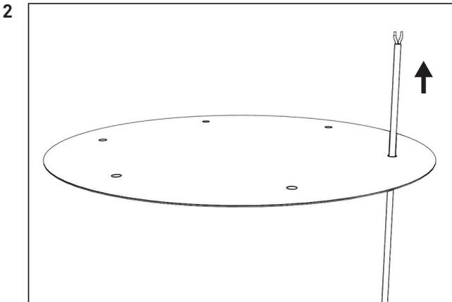
Lead the cables through the cover plate.
