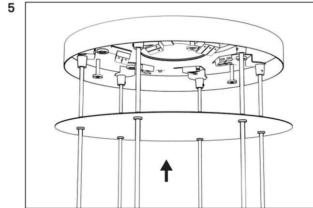
Attach the cover plate to the ceiling plate by carefully sliding it up and let the magnets fixate the cover plate to the ceiling plate.
