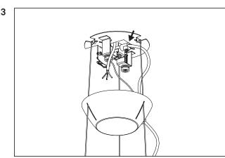
Pull the lamp cable through the cover plate and the strain relief.
