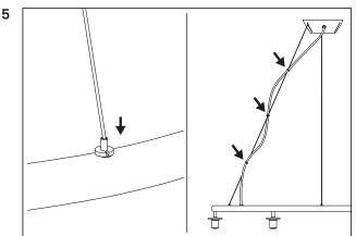
Put the suspension wires into the wire-locks on by one.
