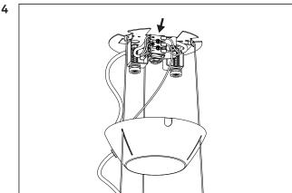
Connect the wire-ends of both the power cable and the lamp cable to the cable terminals. Match the brown wire with "L" the blue wire with "N" and the green/yellow wire with the grounding symbol.
