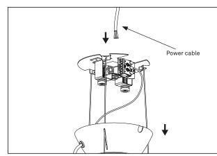
Pull the cover plate away mounting bracket. It is attached with strong magnets and might require some force.
