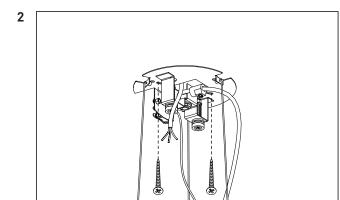
Attach the mounting bracket to the ceiling.
