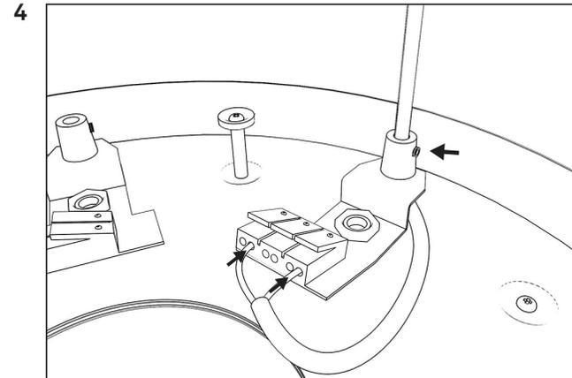
4 Lead the cables through the cable relief and fixate the cable by turning the screw clockwise.
