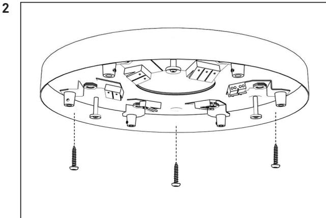
2 Fixate the mounting plate to the ceiling with screws.
