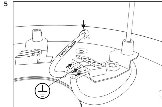
5 Lead the power cable into the ceiling plate and make sure the cable relief is tightened.
