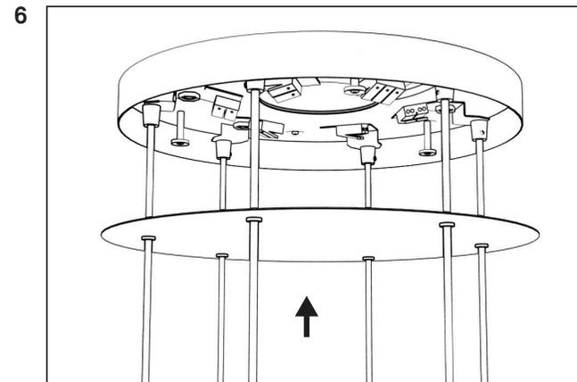
6 Attach the cover plate to the ceiling plate by carefully sliding it up and let the magnets fixate the cover plate to the ceiling plate.
