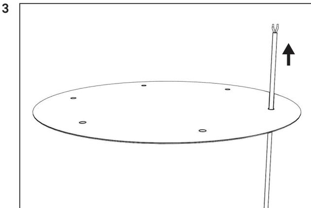
3 Lead the cables through the cover plate.
