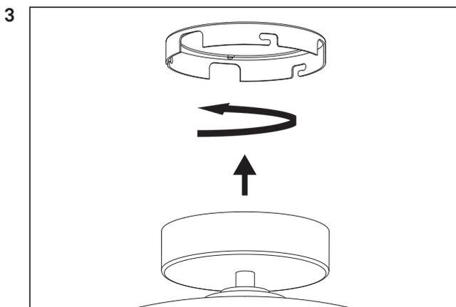
Attach the lamp to the top plate by turning the lamp.
