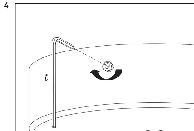
Fixate with the socket screw.
