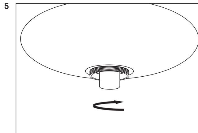
Screw the light bulb into the socket.
