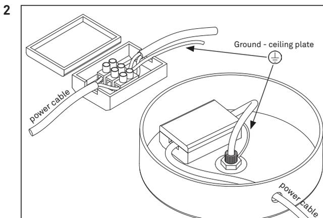
Install the power cable by leading it through either the top or the side of the ceiling plate into the cable connector.
