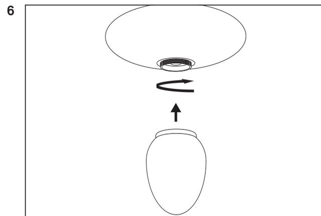
Take the lower glass and carefully place it over the light bulb and socket.
