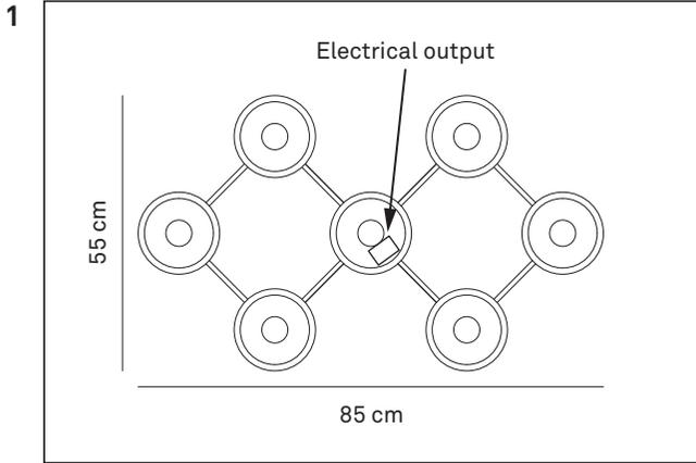
The outer measurements including the cover plates are 85x55 cm.
