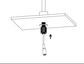
Place the washer and the hand screw over the cable and tighten against the mounting surface.
