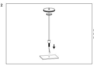
Place the threaded part in the bottom of the lamp into the hole.
