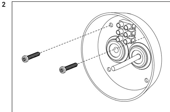
Mount the wall cup to the wall with screws.
