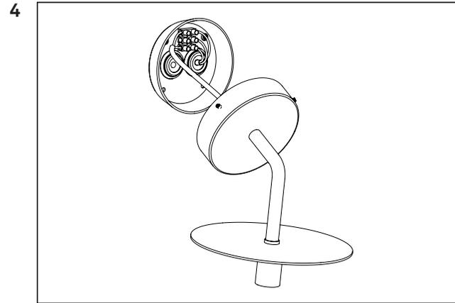
Connect the wire-ends from the lamp to the cable connector.
